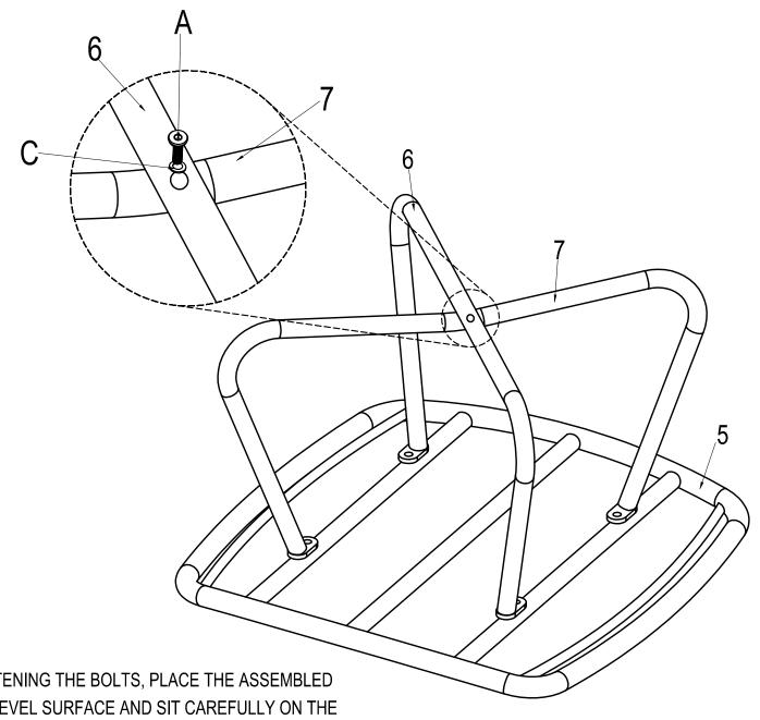
BEFORE FINALLY TIGHTENING THE BOLTS, PLACE THE ASSEMBLED CHAIR UPRIGHT ON A LEVEL SURFACE AND SIT CAREFULLY ON THE CHAIR TO ENSURE THE CHAIR LEGS ARE ALIGNED AND LEVEL. THEN TIGHTEN ALL BOLTS AND YOUR CHAIR IS READY TO USE.
